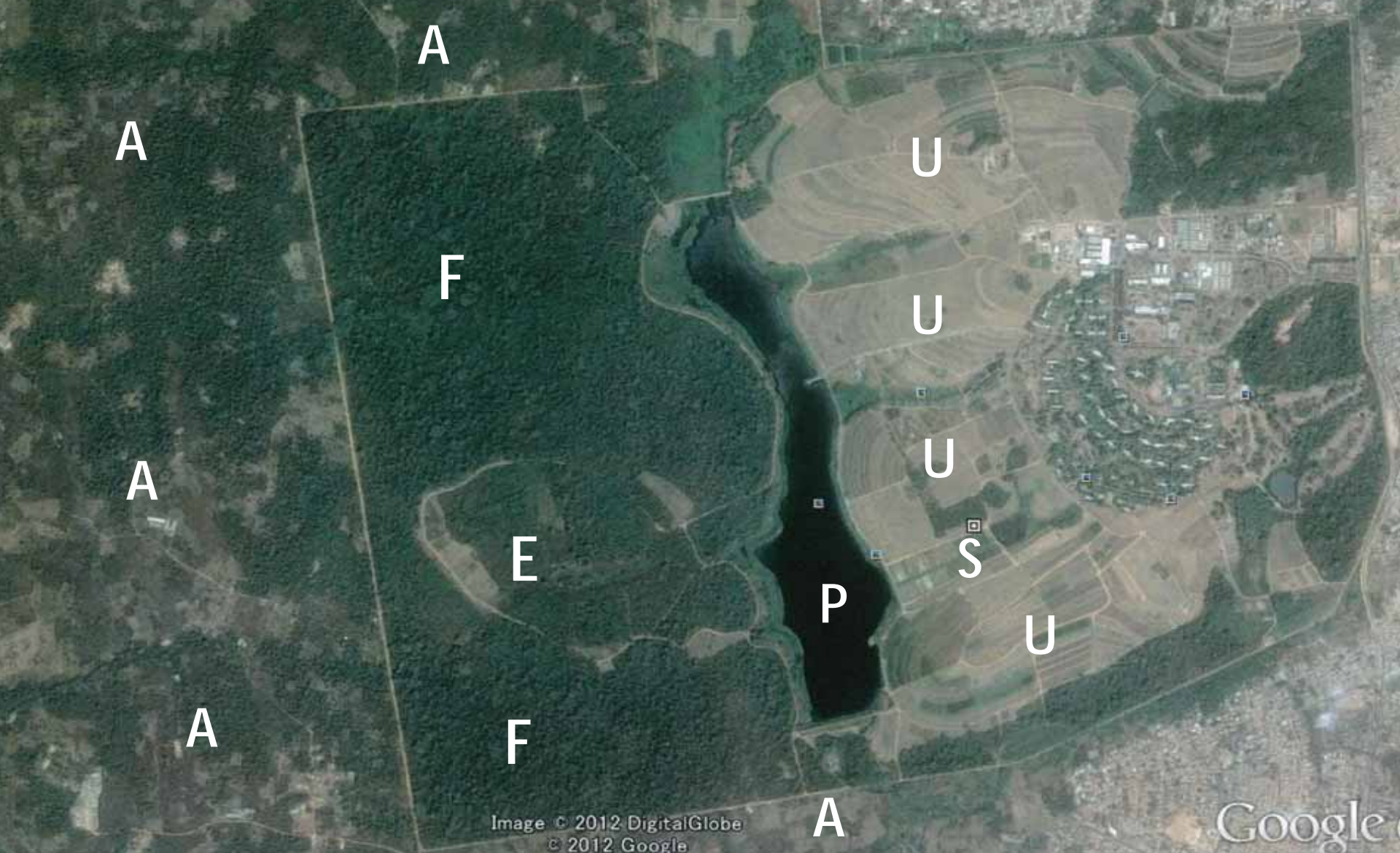
Fig.6. Sawah Hypothesis (1). Prerequisite platform to apply green revolution technologies exist in fenced 1000ha of IITA's research fields, but no such infrastructures farmers' fields. A: Farmers fields with the same soils, topography and hydrology. U: demarcated upland fields along contours. S: Sawah fields at valley bottom. P: Pond for irrigation. F: Regenerated forest, E: Erosion experiment site by Prof. R. Lal and his team in 1970-80s
