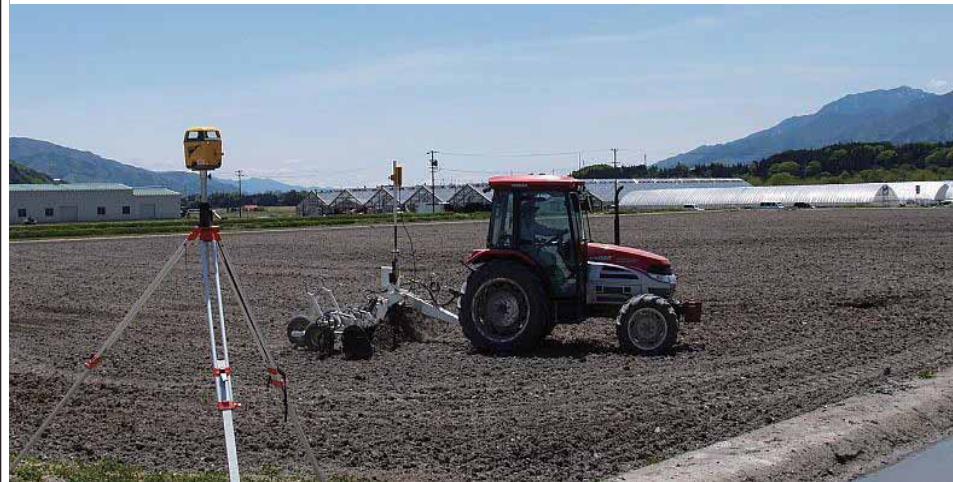
6 th Stage: Advanced and large sawah plot of >1\text{ha} with leveling quality of \pm 2.5\text{cm} using laser leveler tractor (Kubota Co)
