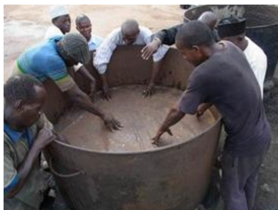
Figure 6: Placement of the false bottom
